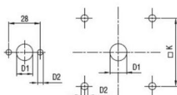
Drillings for 4 screws fixing (4V version).
