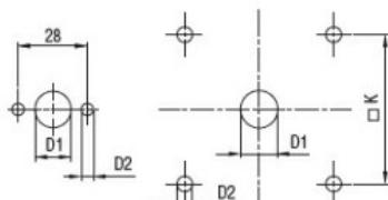
Drillings for 4 screws fixing
