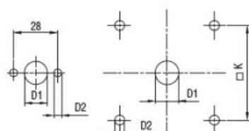
Drillings for 4 screws fixing
