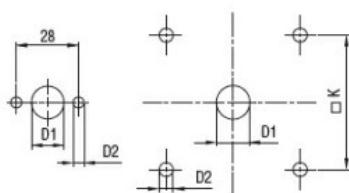
Drillings for 4 screws fixing (4V version).
