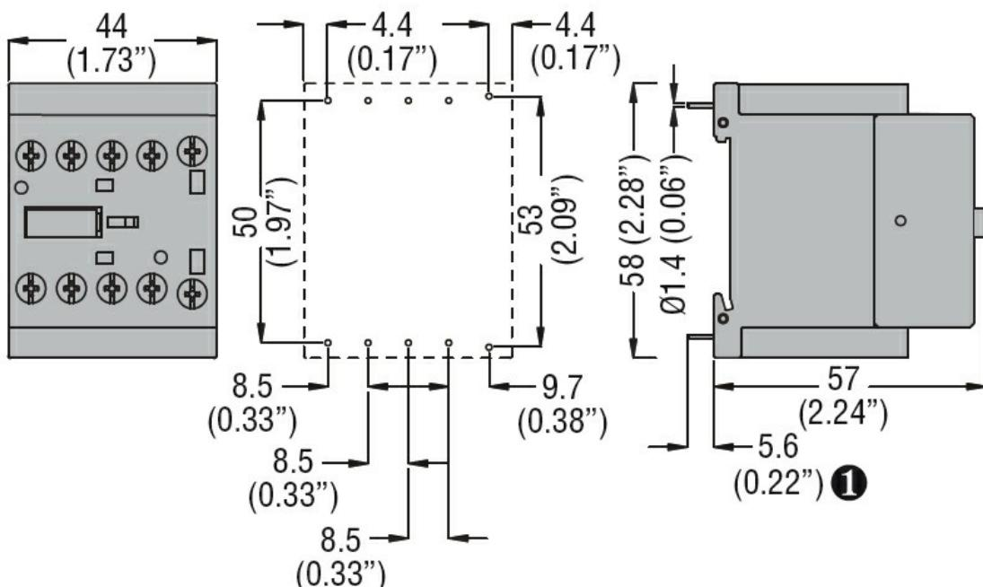
① Recommended PCB drillings 1.7-2mm.
