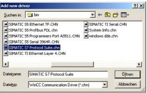
6. For a proper working communication with the PLC there must be defined how the software has to communicate with the PLC
