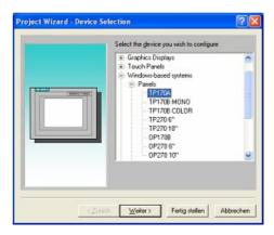
4. "Next" leads you to a new dialog. Type in the specfic fields the name of the PLC device and choose the used PLC in the driver selection (e.g. "SIMATIC S5 – AS511 V6.0")
