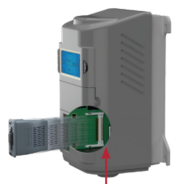
Anybus slot and 50-pin CompactFlash connector on the PCB of the host device
