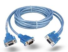
The CAN Y cable can be used to easily loop through CAN or CAN FD networks. It is 2.1 m long, shielded and has twisted wires.
