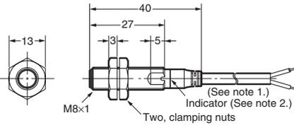
Note 1. 4-dia. vinyl-insulated round cable with 3 conductors (conductor cross section: 0.3 mm<sup>2</sup>; insulator diameter: 1.3 mm); standard length: 2 m
