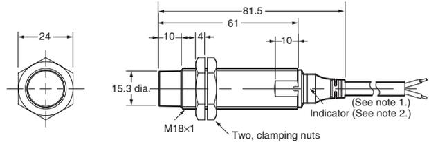
**Note 1.** 4-dia. vinyl-insulated round cable with 3 conductors (conductor cross section: 0.3 mm<sup>2</sup>; insulator diameter: 1.3 mm); standard length: 2 m
